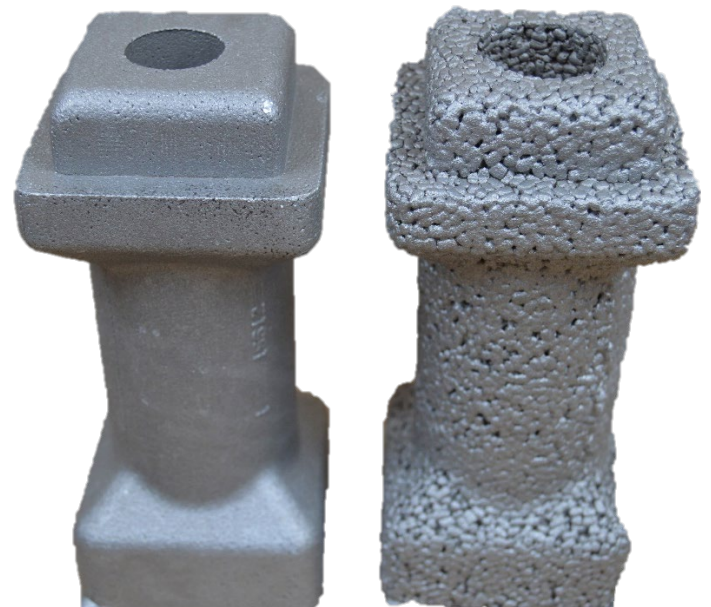
Figure 12. Image of horizontally cast aluminum parts. EPS (left) and EPLA (right).
