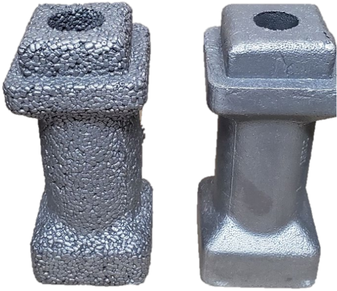
Figure 13. Image of vertically cast gray iron parts. EPS (right) and EPLA (left).
