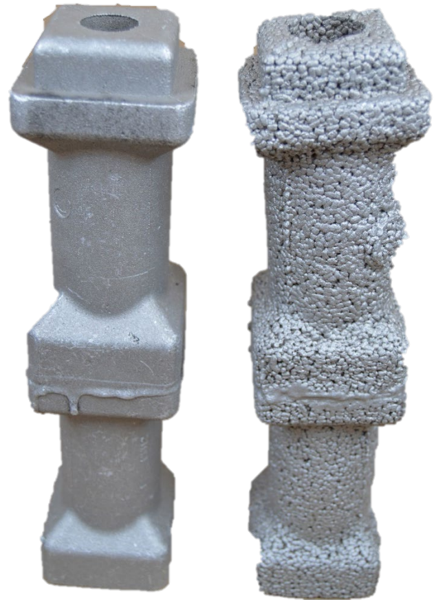
Figure 11. Image of vertically cast aluminum parts vertical casting orientation with two patterns glued on top one another. EPS (left) and EPLA (right).
