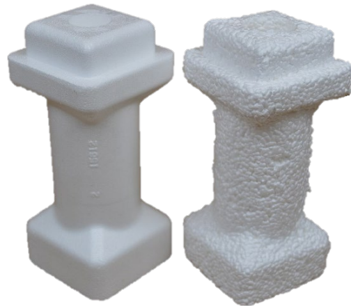
Figure 5. Molded test object (Figure 4) patterns in EPS (left) and EPLA (right).
