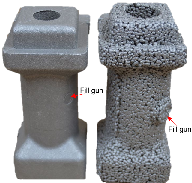
Figure 10. Image of vertically cast aluminum parts. EPS (left) and EPLA (right).
