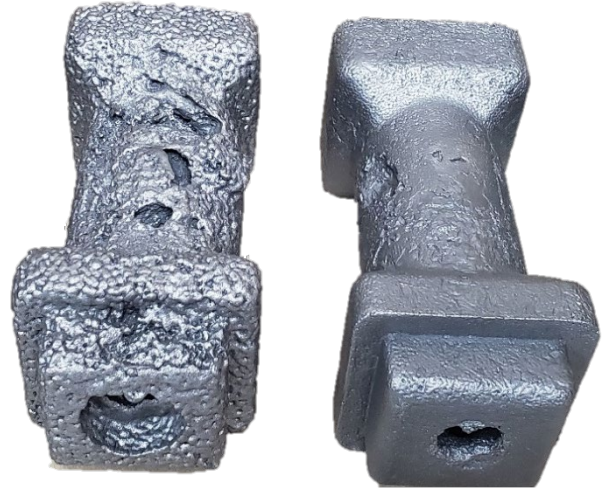
Figure 15. Image of horizontally cast gray iron parts. EPS (right) and EPLA (left).
